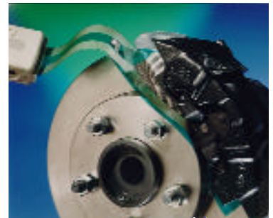
Brake Pad/Rotor Surface Pressure Distribution
