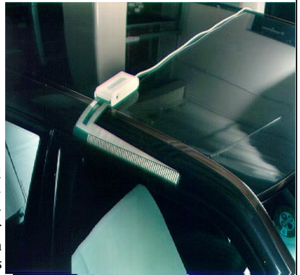
Figure 1. The I-Scan sensor placed between the vehicle door and the rubber door seal.
