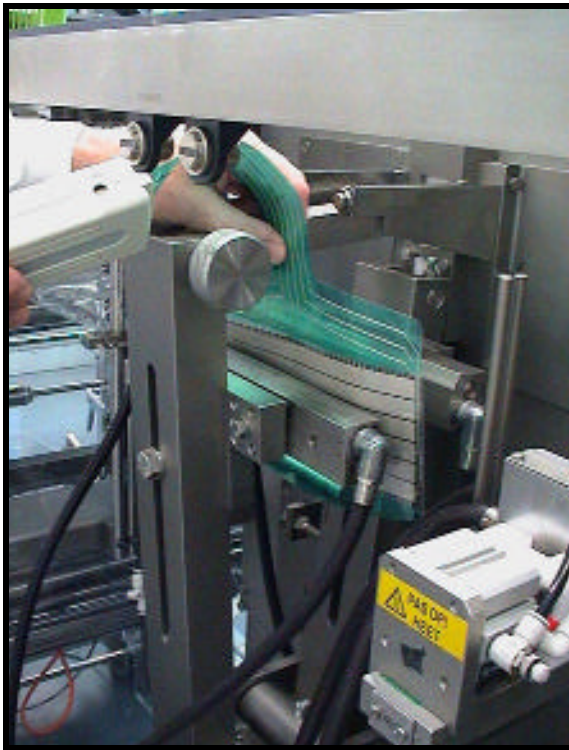
Figure 1 - I-Scan sensor placed between sealing jaws
